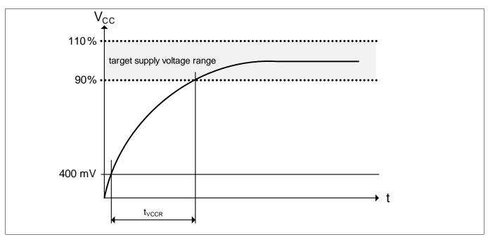
Figure 5 Vcc ramp-up
