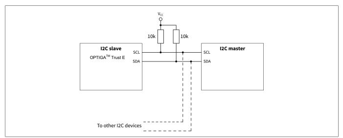
Figure 2 I2C schematic diagram
